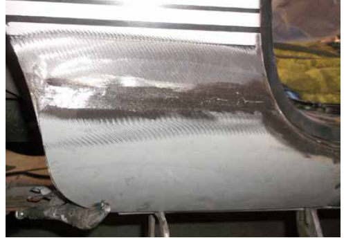
the repaired rocker panel
