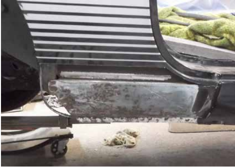
Rust cut out of rocker panel
